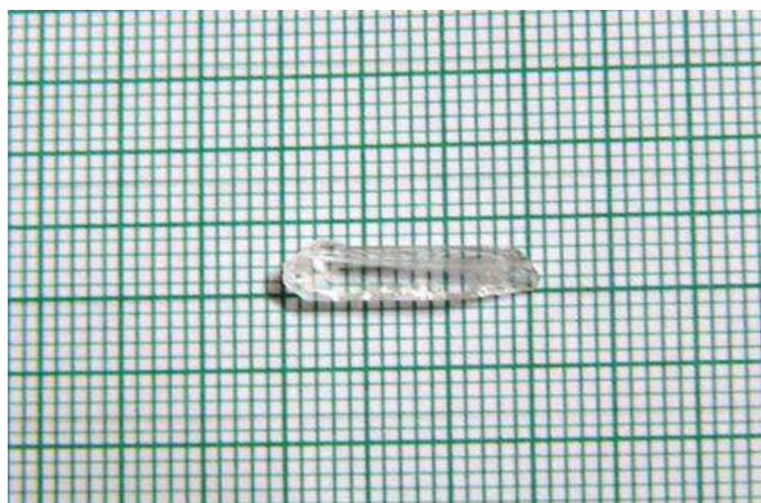
Fig.1. As-grown single crystal of GGC
