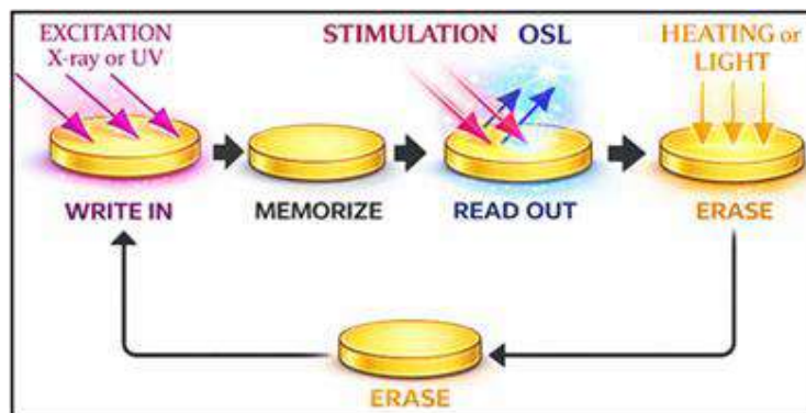
Fig. 2: Schematic representation of the OSL process showing the stages of energy storage and release.
