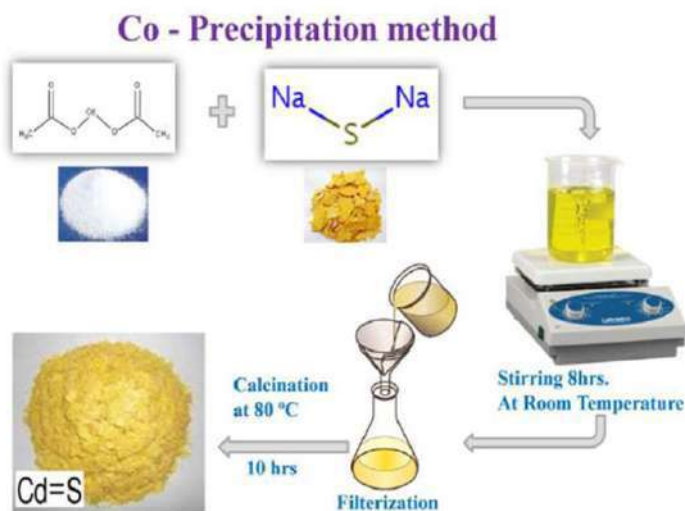
Fig.2: A flow chart Diagram of synthesis of CdS Nanomaterial
