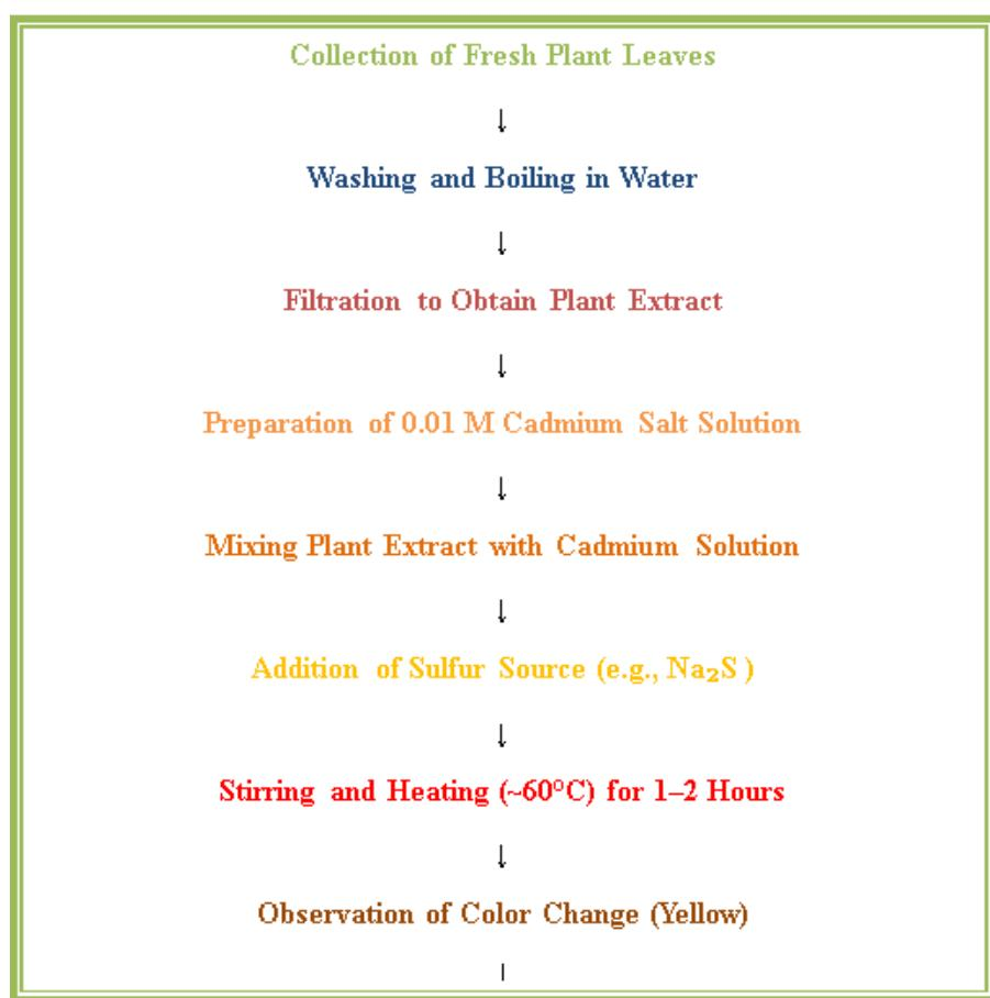
**Fig.1: Flow chart of CdS nanoparticles using Green Synthesis method**
