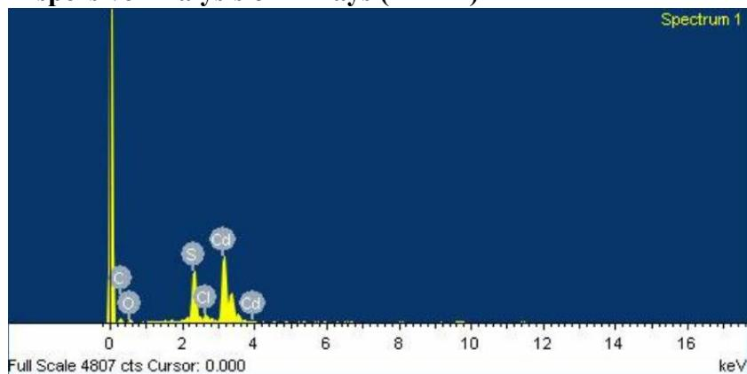
Fig. 4: EDAX spectrum of CdS nanoparticles
