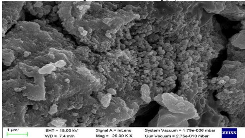
*Fig. 2: SEM micrograph CdS nanoparticles*
