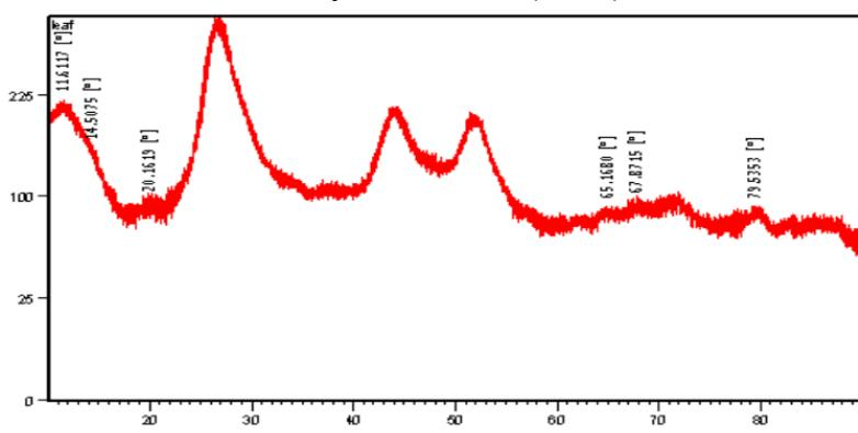
Fig. 3: XRD spectrum of CdS nanoparticles [12]
