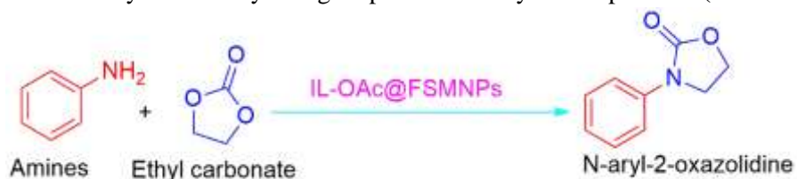
Scheme 7. Synthesis of N-aryl 2-oxazolidinone derivative catalyzed by IL-OAc@FMSNPs nanoparticles
