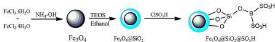
Scheme 8. Synthesis of sulfated boric acid supported silica-coated nanoparticles
