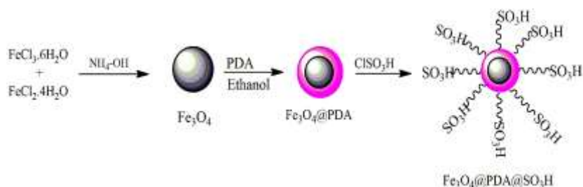
Scheme 4. Synthesis of Polydopamine chlorosulfonic acid supported silica-coated nanoparticles
